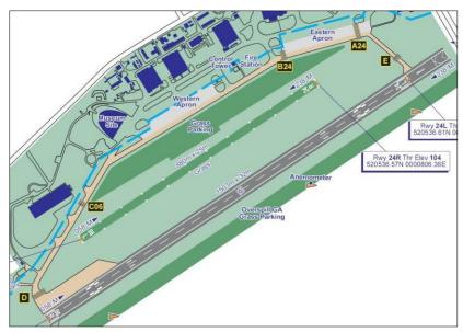
**Departures to the north: RWY 24** -climb straight ahead for 5nm or at and above 2,000ft before turning north **RWY 06** - climb straight ahead for 2nm before turning north
