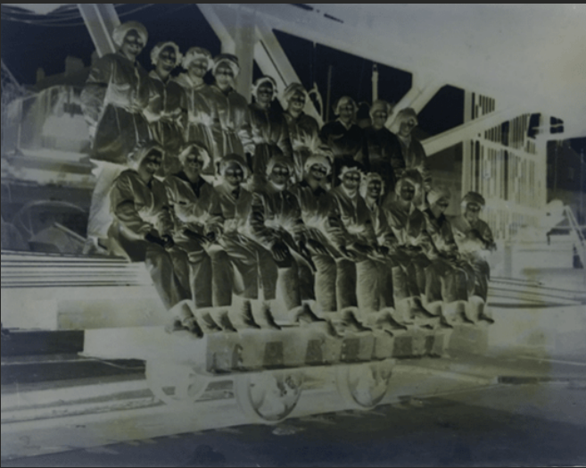
Glass plate negative showing degradation which is being given remedial conservation treatment.
